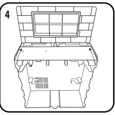
Fit the rear shell upper cover to the rear shell. Noted: the left and right sides should be aligned and inserted.
