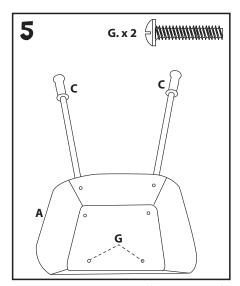
Insert two Large Screws (G) into the openings on the inside of the Wheelbarrow and through the openings on the Leg Supports (B1, B2).
