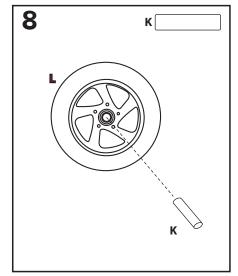
Insert the Bushing (K) in to the center opening of the wheel.
