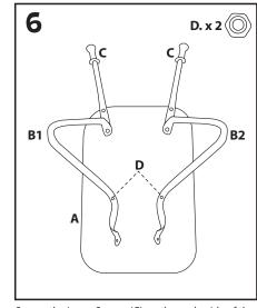
Secure the Large Screws (G) on the underside of the Wheelbarrow using two Small Nuts (D).
