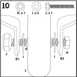
Insert one Bolt (J) through the Left Lea Support (B1). Then, place one Large Washer (I) over the bolt. Slide the Bolt through the Bushing (K) in the Center of the Wheel (L). Slide another Large Washer (I) over the Bolt. Place the end of the Bolt through the Right Leg Support (B2). Hold the Bolt with one wrench, and secure the assembly with the Large Nut (H) using another wrench.
