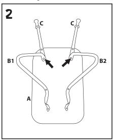
Position the Left Support Leg (B1) and Right Support Leg (B2) under the Wheelbarrow (A) so that the openings align with the lower openings on the handles (C). The legs should bow outward.
