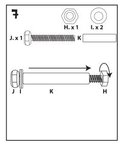
Remove the Large Nut (H), Bushing (K), and two Large Washers (I) from the Large Bolt (J).
