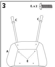
Insert two Small Screws (E) into the openings on the inside of the Wheelbarrow and through the openings on the Leg Supports (B1, B2) and Handles (C).
