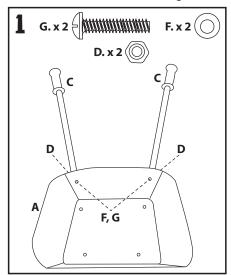
Align the Handles (C) with the openings on the back of the Wheelbarrow (A). Slide a Small Washer (F) onto both Large Screws (G). Insert the screws into the openings on the inside of the wheelbarrow and through the openings on the Handles (C). Secure the screws on the backside of the Handles using two Small Nuts (D).
