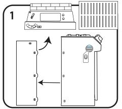
Pull out the back wall of the oven and remove the top panel and shelf. Then, remove and discard the tape holding the cookie sheet to the oven's door to
