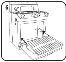
To insert the shelf, slide the sides of the shelf in between the brackets in the oven.
