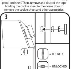
Insert a screw on each side of the top panel and turn the screw to lock in place. The screw should enter both openings.
