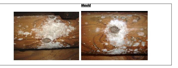
Mould growth is a natural process on the surface of wood, especially when stored in dark, damp, warmer conditions with poor ventilation. It is easily removed with a stiff bristled brush and, if necessary, soap and hot water. We do not ship wood that shows an initial mould condition, but the growth of mould may continue over time, even after shipment, due to the wood's natural reaction to the aforementioned conditions.
