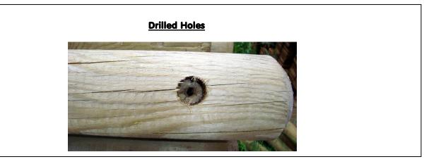
The wood is provided to you with some holes pre-drilled. Although drilling wood is a controlled process, the outer finish of drilled holes will vary depending on the density and certain characteristics specific to each piece of wood.
