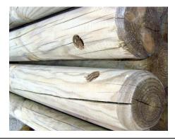
Wood will split or crack due to changing climate and moisture fluctuations in the environment. In round wood, these cracks are acceptable up to 5mm wide and 30% of the depth of the diameter, even when they run along the length of the wood. This will not affect the strength of the pole.
